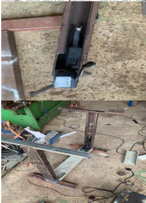
Figure2: Linear actuator with a table arm
